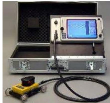
Radar scanning survey equipment
